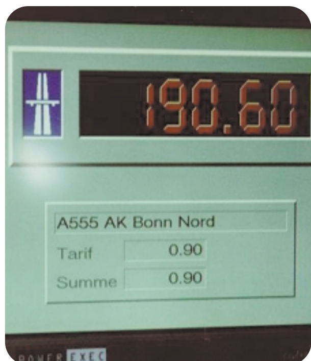
Screen from the Mannesman’s ROBIN system using GPS to define virtual road-charging payment locations. Courtesy Oscar Faber.
