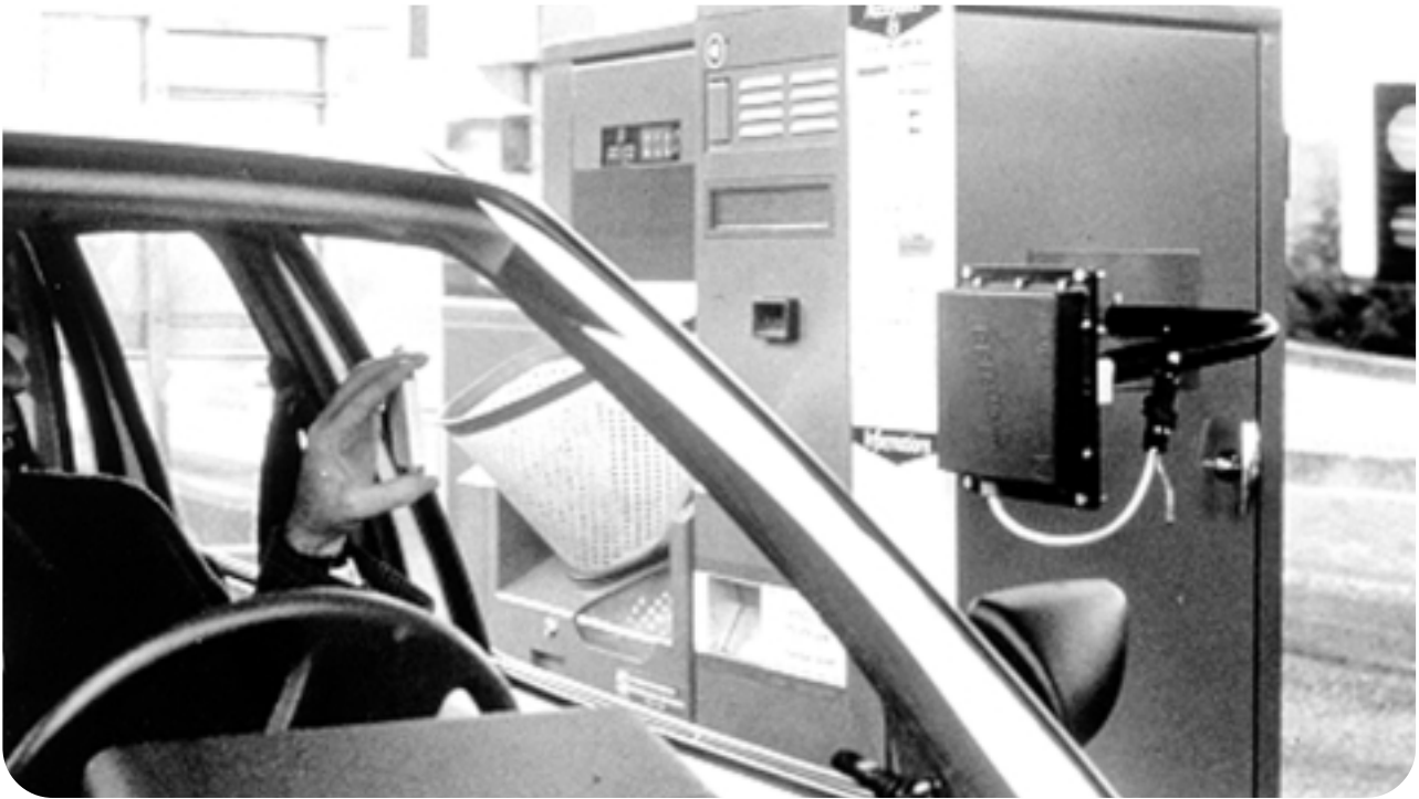
Smartcard and roadside automatic debiting equipment. Courtesy Oscar Faber.
