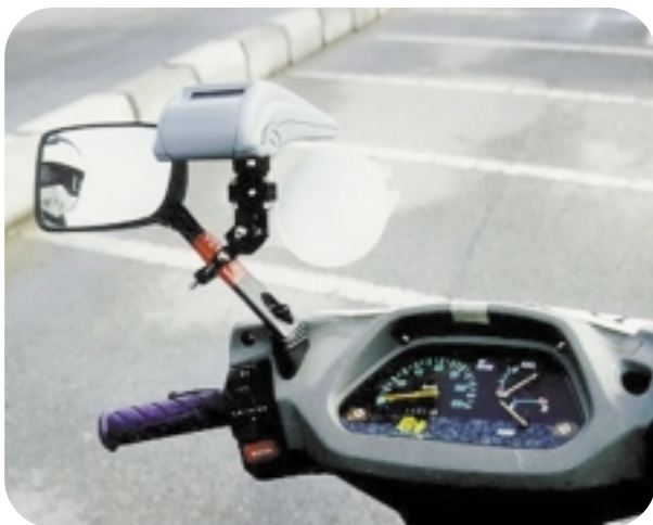
Waterproofing housing for transponder mounted on motorbike from CEC-SEEL trial in Singapore. Courtesy Oscar Faber.
